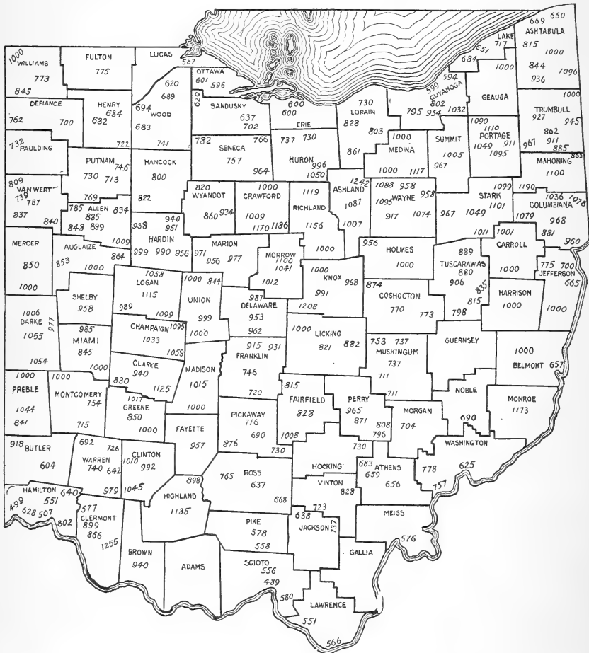
FIG. 4.—Map of Ohio, giving elevations at various points as determined by railway surveys (original).
